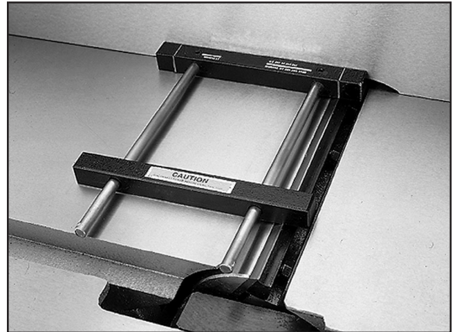
Figure 36. G1753 Jointer Pal® Knife Gauge.
